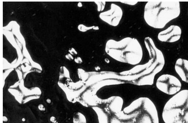
Figure 8 Photomicrograph of LCPA-03 at 242°C (crossed polarizers; original magnification, 360 \times ).
